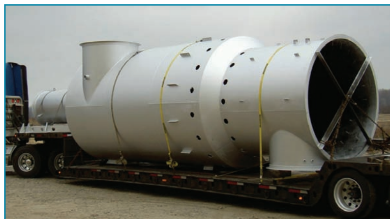
A low NO x Oxidizer is transported by truck to the Howard City, Mich. Waste-to-Energy site being built by Heat Transfer International.
