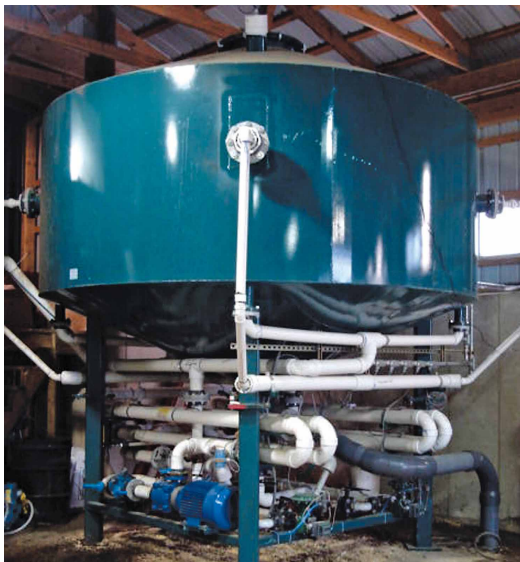
Digester effluent exiting the system goes through an auger screw press separator (top). The solids, or biofibers, are densified into pellets. The liquid portion of the effluent is run through a dissolved air flotation process (bottom) to separate out suspended solids.
