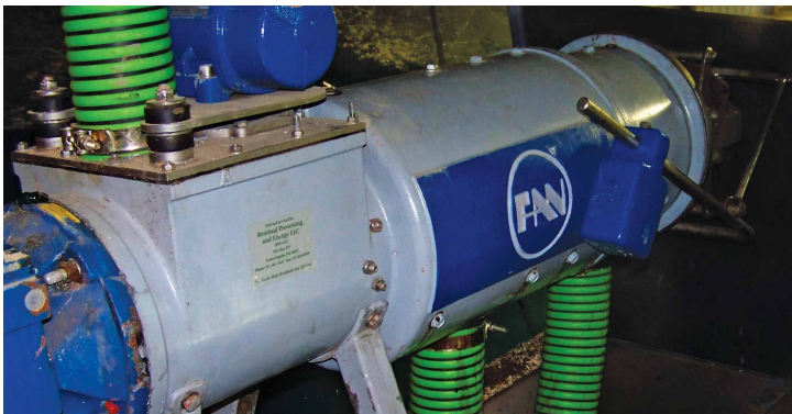
Digester effluent exiting the system goes through an auger screw press separator (top). The solids, or biofibers, are densified into pellets. The liquid portion of the effluent is run through a dissolved air flotation process (bottom) to separate out suspended solids.
